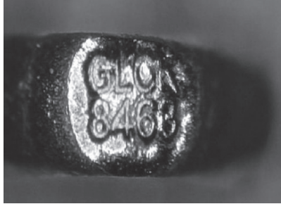
A study by Lucien Haag presented to the National Academy of Sciences featured this Glock firing pin after 1400 rounds (image reversed).
